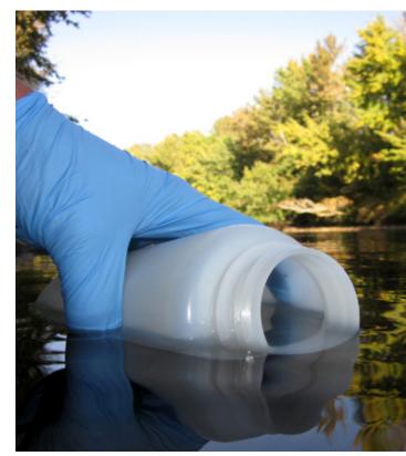
For the most reliable results, water samples should be kept cool, in the dark, and delivered to the AWRC Water Quality Lab as soon as possible.
