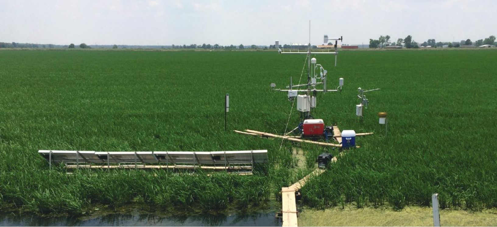
Image caption: Eddy covariance tower deployed at a rice field in Arkansas.
