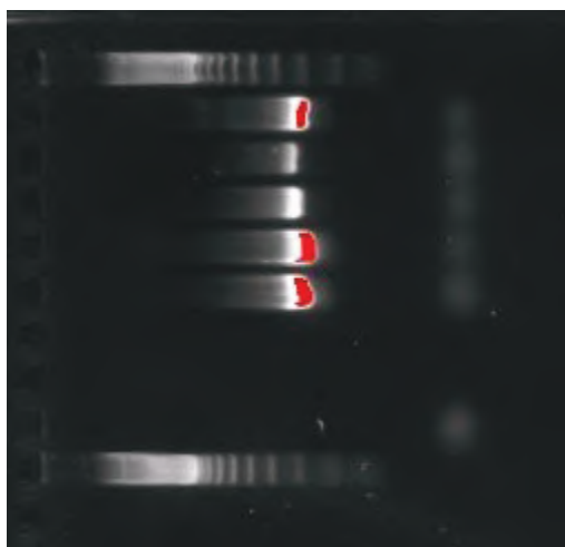
Figure 5: Gel electrophoresis image showing the successful amplification of DNA extracted from biofilms in the pipe samples from the pipe loop on March 22, 2017. The wells contain: ladder, 5 DNA extracts from Galvanized Steel, Copper Type K, Lead, PEX-A and PVC pipes, negative control, and ladder (in vertical order).
