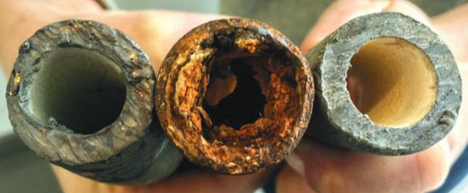
Image caption: Biofilms accumulate inside drinking water distribution pipes.
