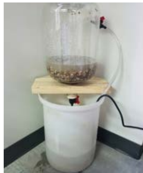
Figure 1: Example of the pump-included hydroponic wastewater system.
