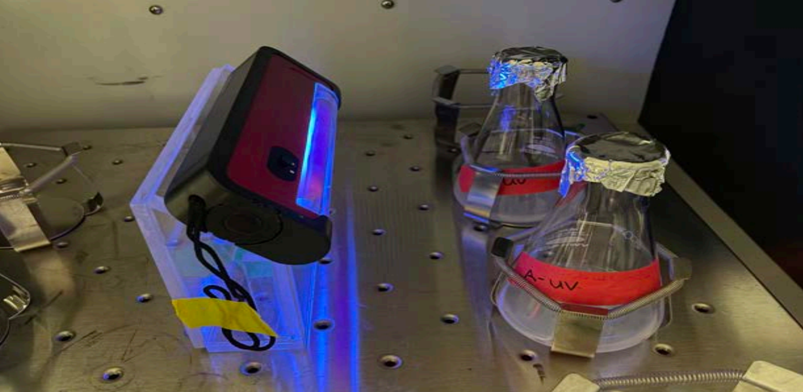
Image caption: A glimpse into the general experimental setup utilized. Flasks containing MC-LR, \text{TiO}_2 , and DI water are exposed to UV light while being mixed. Normally, this is covered as to not allow outside light to interfere with the UV treatment. Photo courtesy of Zane Wood.
