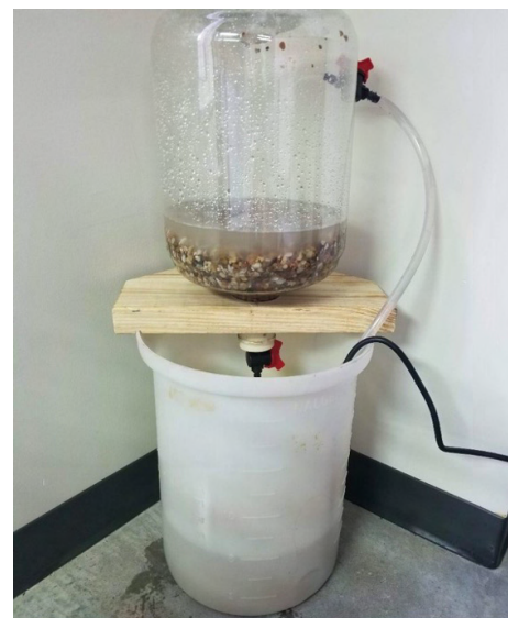
Figure 1: Example of the pump-included hydroponic wastewater system.
